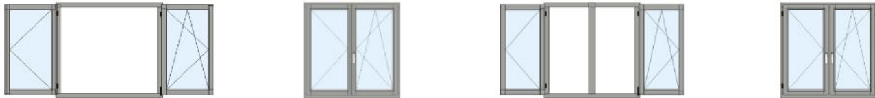
window with floating mullion, opened window with floating mullion, closed window with a fixed mullion, opened window with a fixed mullion, closed
